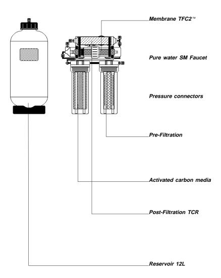
made of a exclusive Thin-Film C2 composite that offers higher rejection, greater structural stability, operates more effectively at lower pressures and will produce more water faster than other earlier types of membrane.
